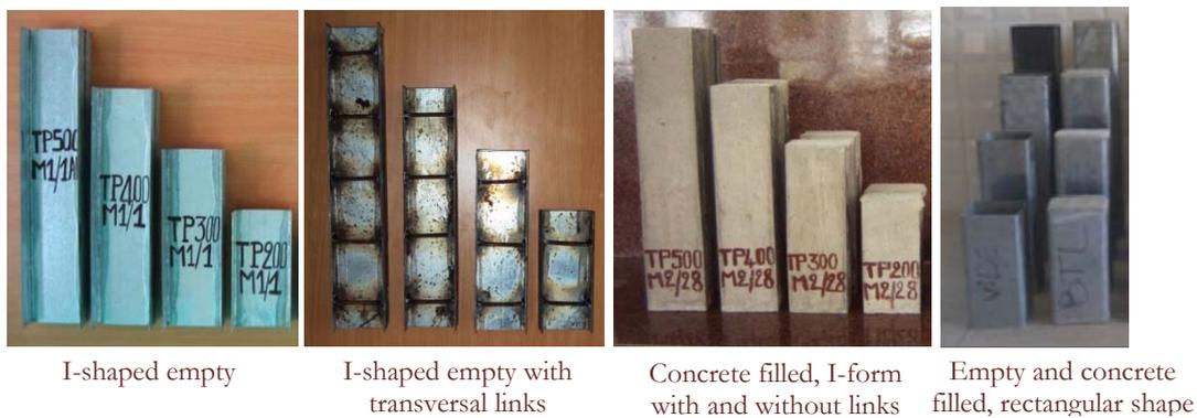
Figure 2: A general view of the fabricated specimens.
