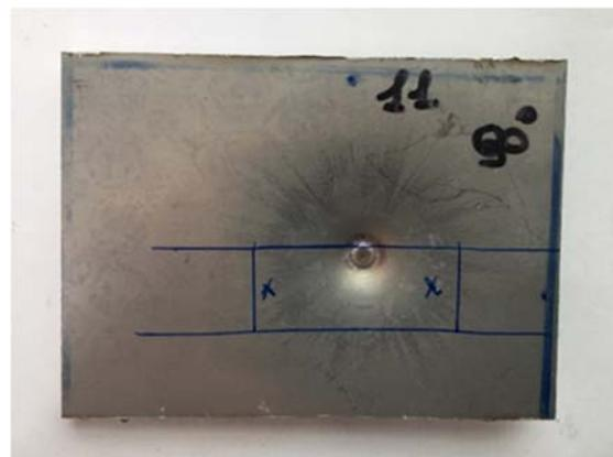
Figure 11: Sample cut for micrographic analysis.
