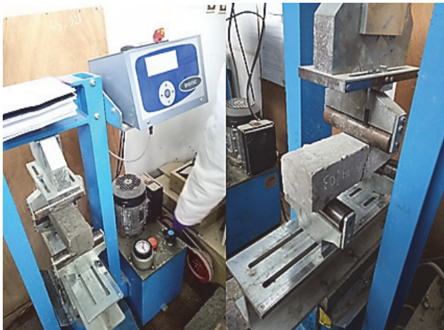
Figure 2: Tensile machine, three point bending test.
