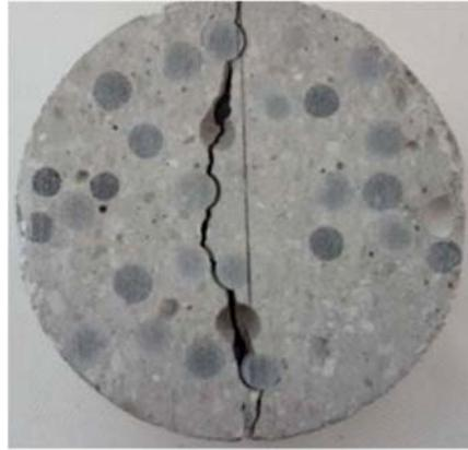
Figure 11: Crack's path obtained during the splitting tensile test [21].
