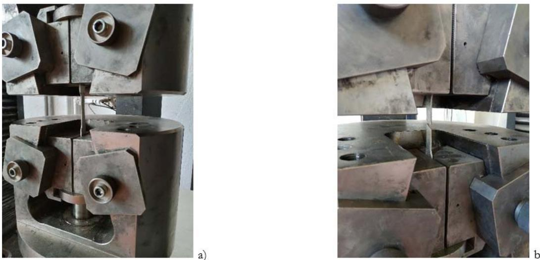
Figure 8: Detail of tensile test execution: a) Specimen before the start of the test; b) Specimen at the end of the test.
