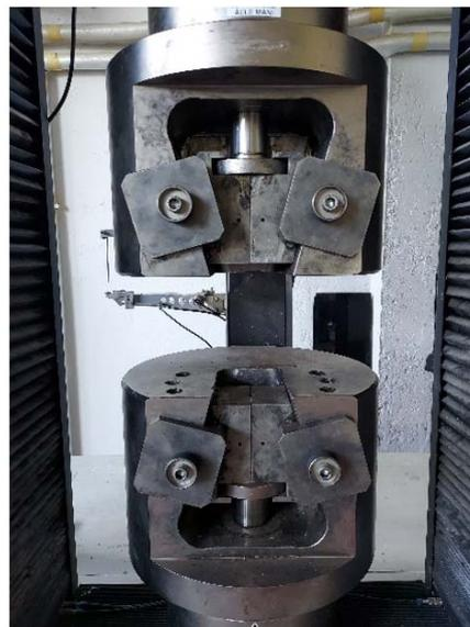
Figure 7: Tensile testing machine detail.
