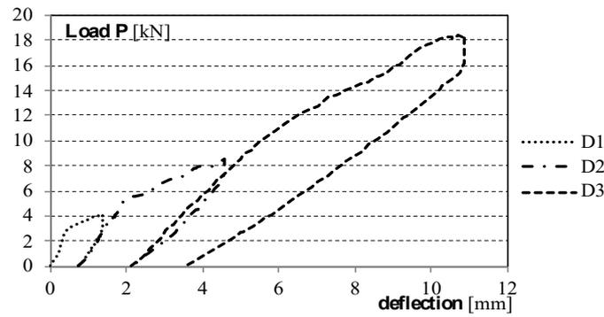
Figure 10: Load-Deflection diagrams for the first three damage level on un-strengthened RC beam B2.
