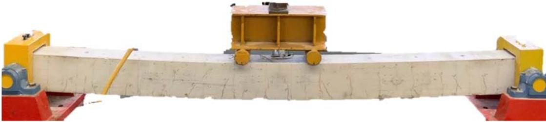
Figure 13: Visualization of cracks by bending loading at damage level  $D_4$  for RC beam B2 strengthened with NSM GFRP rod.
