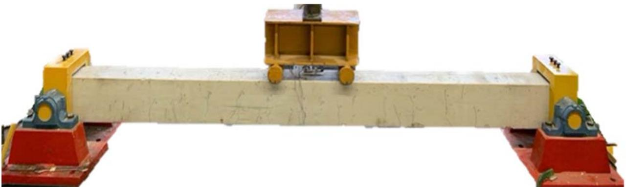
Figure 8: Visualization of cracks by bending loading at damage level  $D_3$  for RC beam B1 without strengthening.
