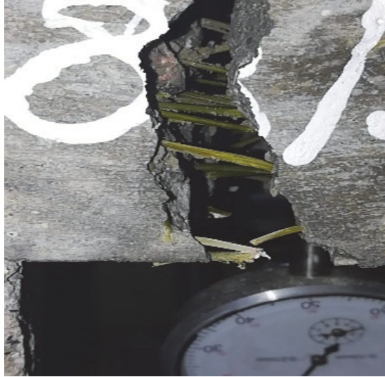
Figure 14: Resistance of Alfa fibers to crack propagation.
