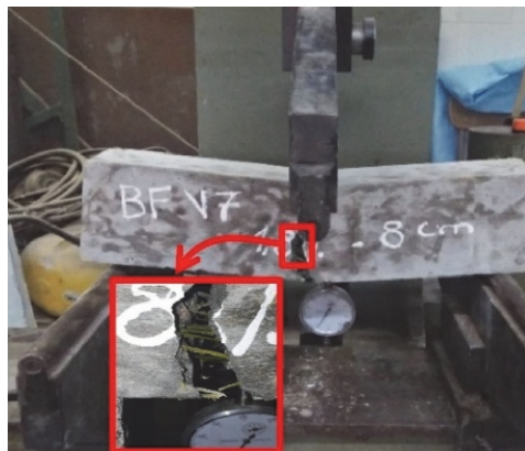
Figure 8: Tensile fracture of Alfa fiber concrete specimen.
