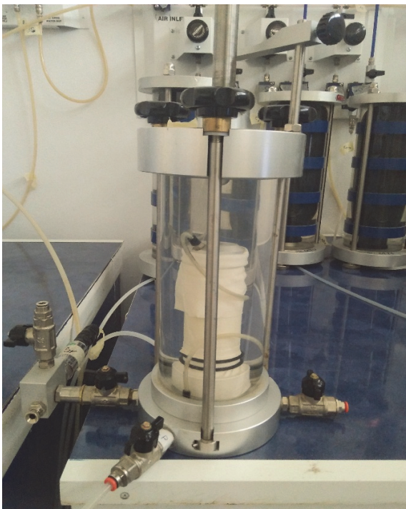
Figure 3: Sand specimen before and after performing the shear test.
