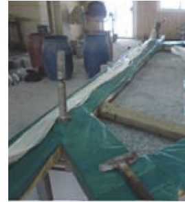
b) Continuous fibers are tensioned between 2 hooks.
