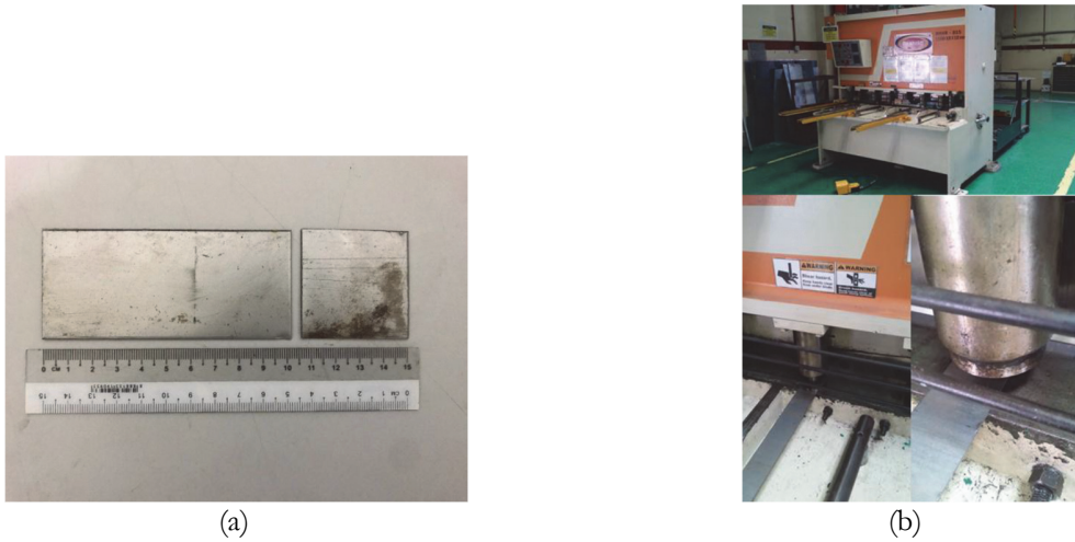
Figure 2: Specimen preparation: (a) Dimension for rectangular and square parts; (b) Shear machine
