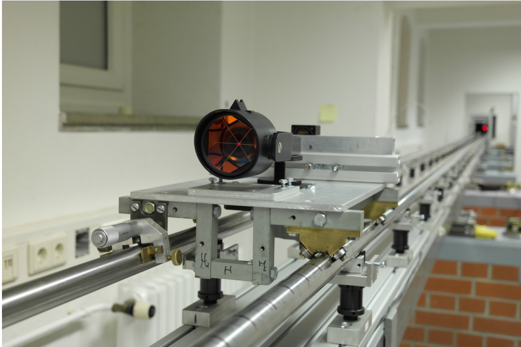
Figure 3: Prism on the laser-interferometer line
