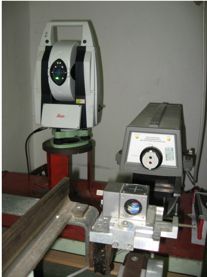
Figure 2: Calibration of the laser-tracker Leica AT401 with use of the laserinterferometer
