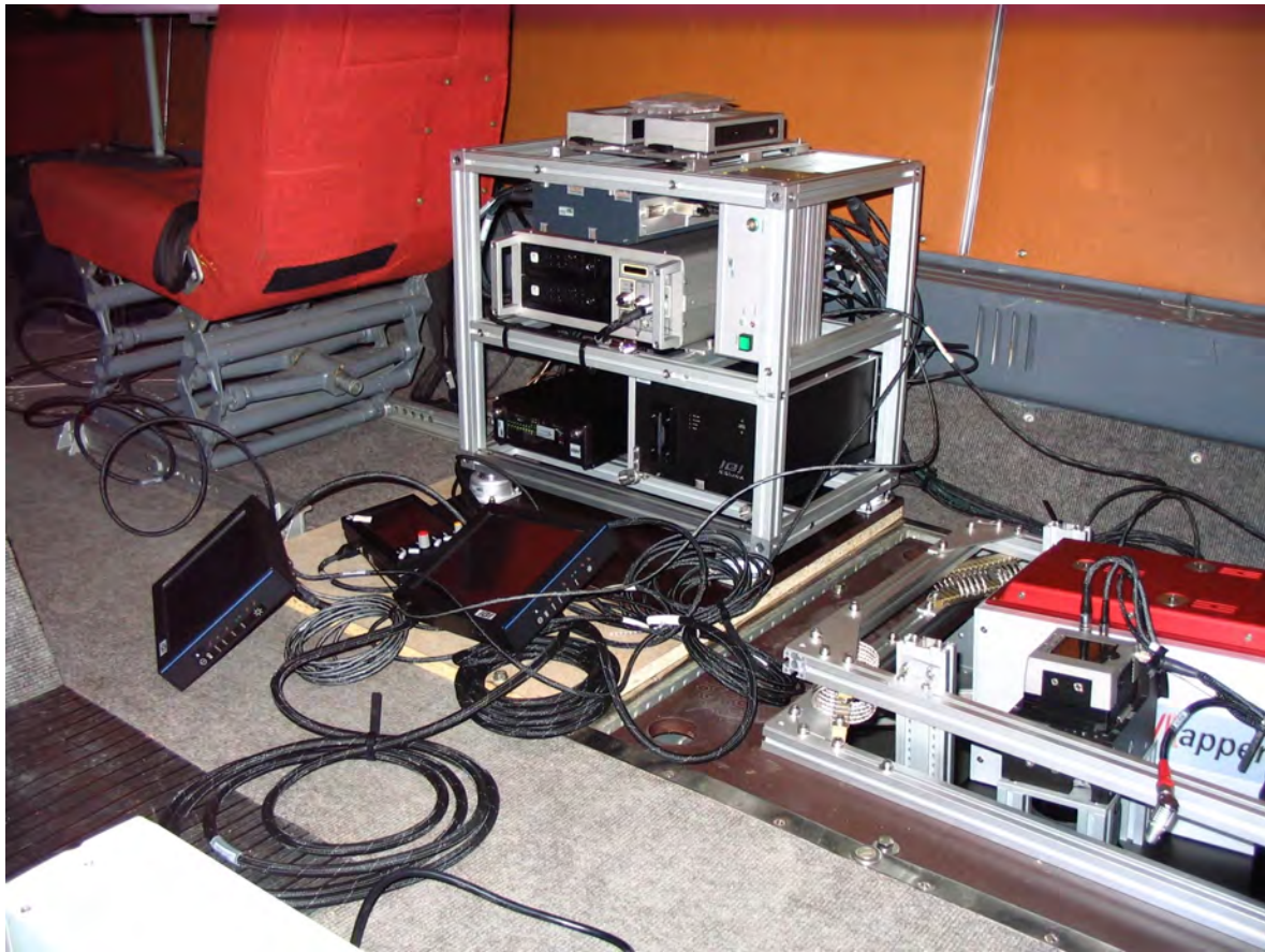
Figure 5: Laser scanning system LITEMAPPER on the board of L-410 FG aircraft
