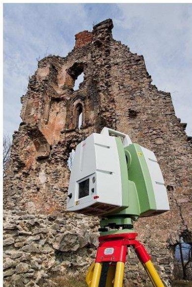
Figure 7: a) Leica ScanStation C10 over a scan station, b) its technical specification
