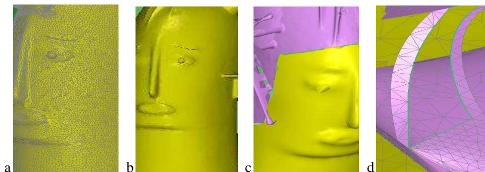
Figure 7: Modelling phases for “Mentoring”: a) Meshing; b) Smoothing; c) Joining parts; d) Holes filling
