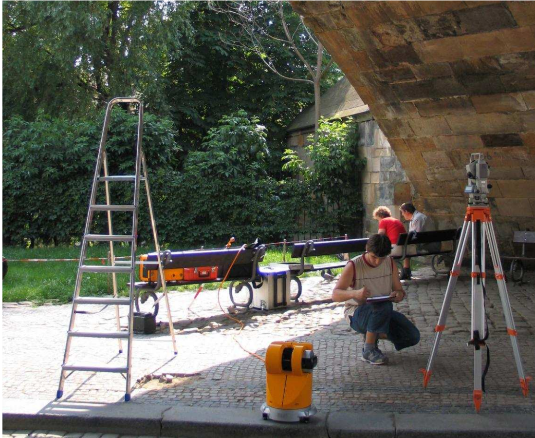
Figure 1: Complex documentation of Charles Bridge vault in Prague obtained by laser scanner Callidus
