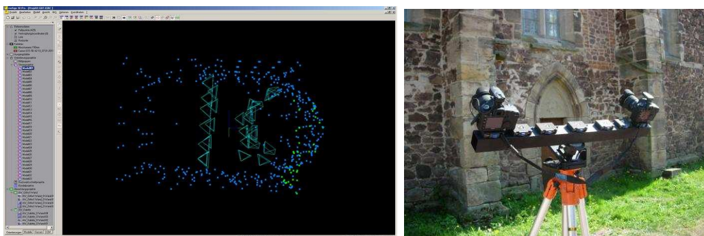
Figure 1: Left: recording configuration at east wall and apse (castle of Katzenstein); right: used recording rail with 2 reflex cameras
