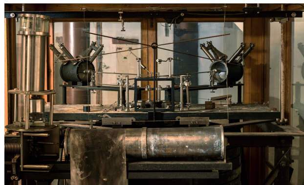
Fig. 2. In COP's Caponière XIII, the purely mechanical Wiechert Horizontal seismograph is still in its original location. Photo: Casper Brogaard Højer.
