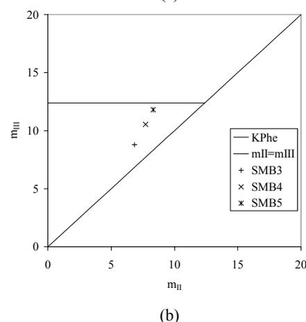
Figure 4. The measurements points placed in the Morbidelli triangle: a) phenylalanine-glycine separation at temperature  $20^\circ\text{C}$  (AA03) and  $60^\circ\text{C}$  (AA06) b) desalting of phenylalanine (SMB 3, 4, 5).
