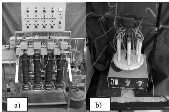
Figure 2. Photography of a) production scale SMB and b) small-lab SMB equipment.
