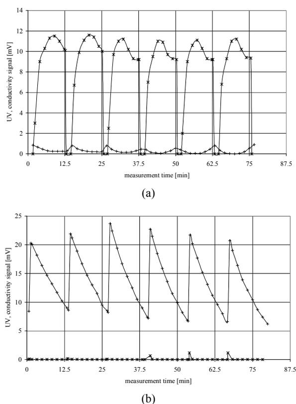
Figure 5. Measured concentration commensurable signals by SMB5 experiment in a) raffinate and b) extract. Markers: signal of phenylalanine (+) and signal of NaCl (\*).
