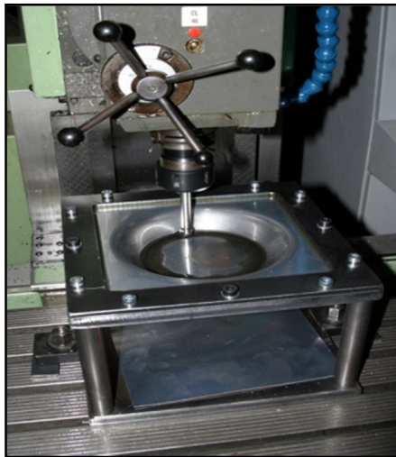
Fig. 1: Incremental sheet metal forming process [4].
