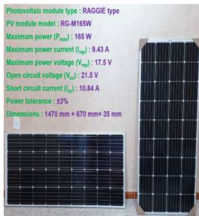
Figure 1. Studied photovoltaic panels and their technical characteristics
