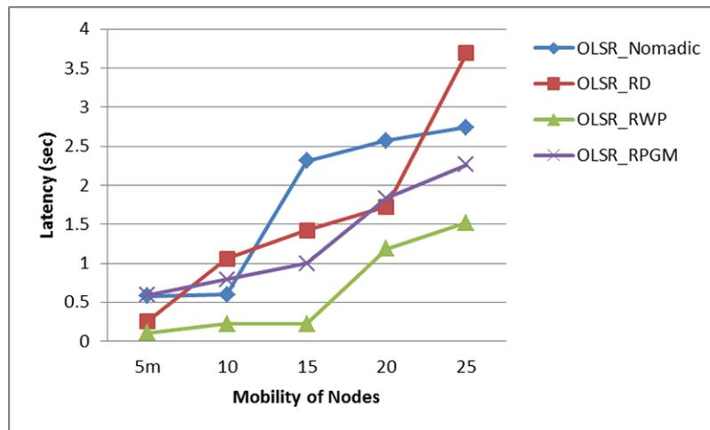
**Fig. 8.** Latency analysis of OLSR under four mobility models with low degree of mobility
