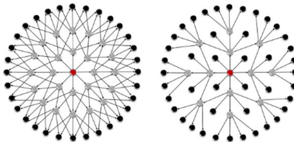
Fig. 6. Optimizing flooding of control traffic in OLSR using MPR
