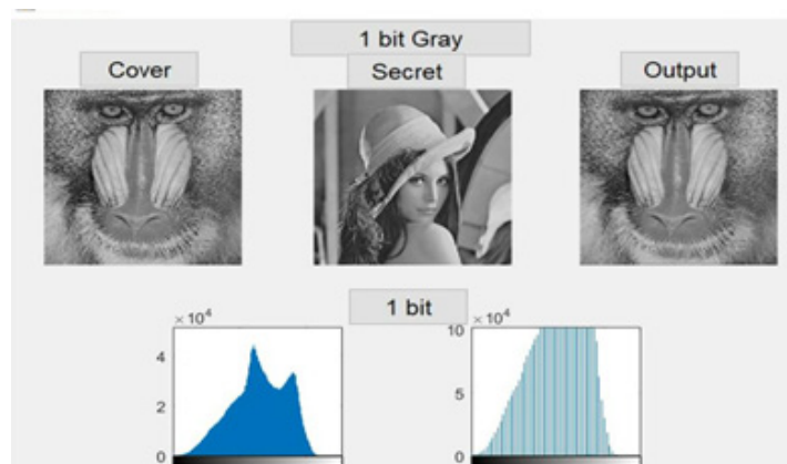
Fig. 5. Grayscale cover and stego image and their histogram using the 1-LSB method
