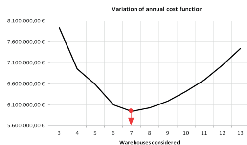
Figure 3. Relationship between the annual total cost and the number of warehouses considered in the model.
