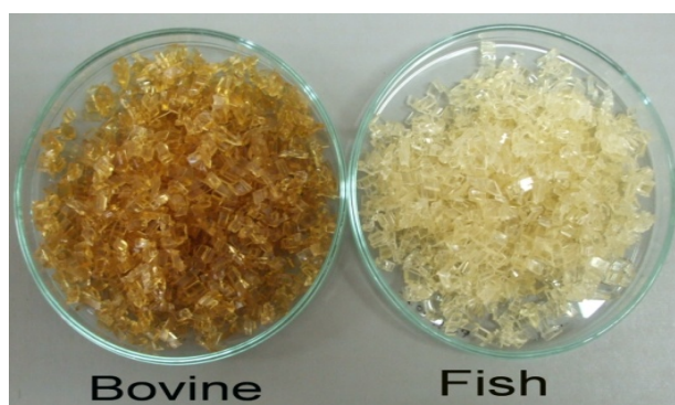
Figure 1. Photographs of molding compound resins from bovine and fish gelatins.
