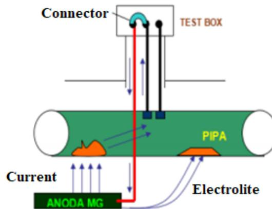
Figure 1. The procedure sacrificial anode system [3]
