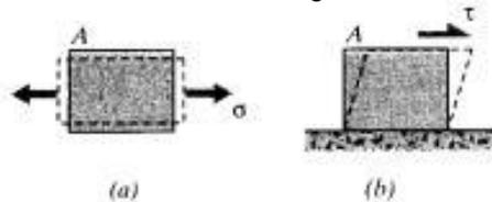
Figure 3. (a) Normal and (b) shearing deformations
