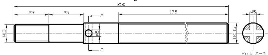
Figure 1. A Screwed Shaft
