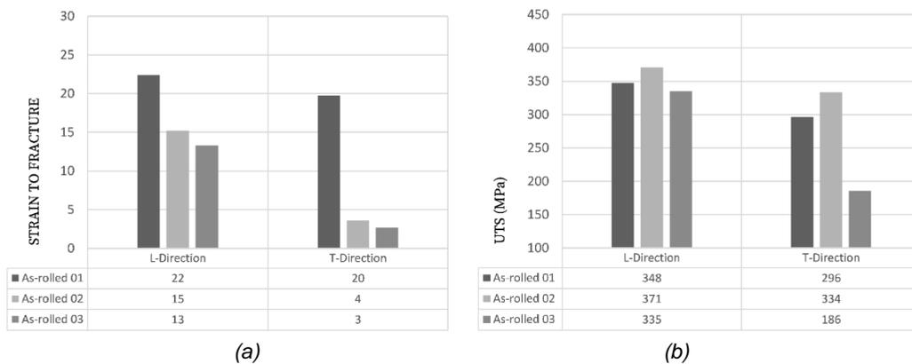
Graphic 1. (a) Strain to fracture values, (b) UTS values as-rolled condition
