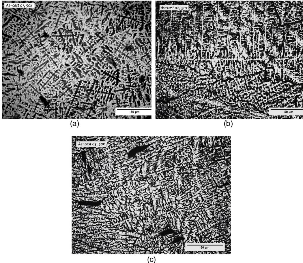
Figure 1. As-cast microstructure of a) Alloy 1, b) Alloy 2 and c) Alloy 3
