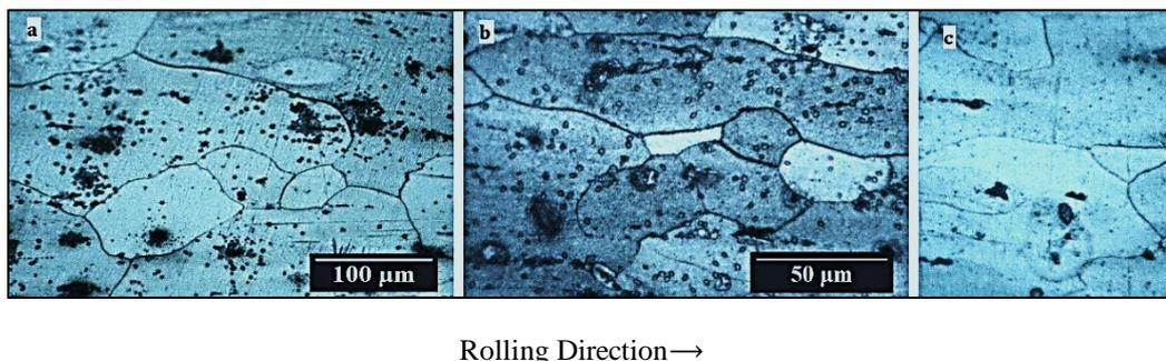
Figure 2. Microstructure of (a) alloy 01, (b) alloy 02 and (c) alloy 03 as-rolled condition
