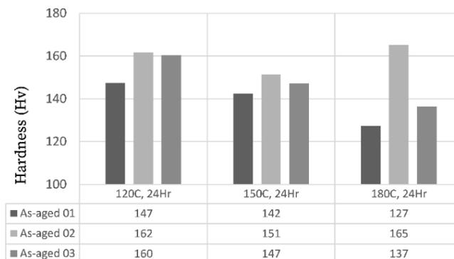
Graphic 3. Vickers hardness for alloys 1, 2, and 3 aged at 120 °C /24 hr, 150 °C /24 hr, and 180 °C /24 hr
