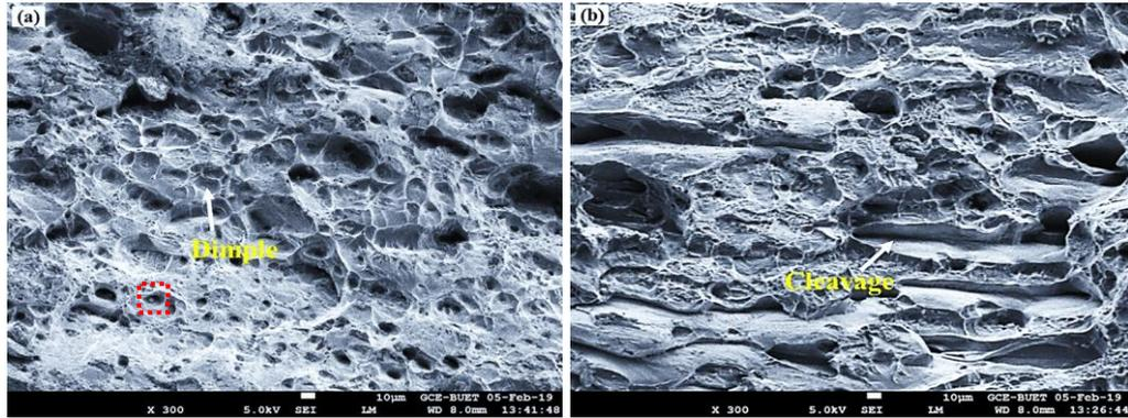
Fig. 7 SEM image of fracture surface along (a) longitudinal- alloy 01, and (b) transverse directions- alloy 02 as-aged at 150<sup>0</sup> C/24hr.
