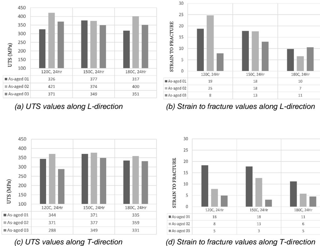
Graphic 2. UTS and strain to fracture values along longitudinal and transverse directions as-aged at different temperature-time cycles
