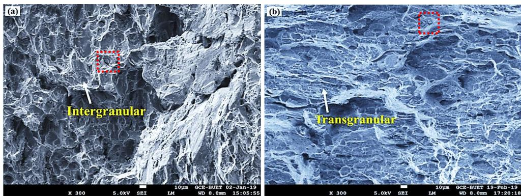
Fig. 8 SEM image of fracture surface along (a) longitudinal- alloy 02, and (b) transverse directions- alloy 02 as-aged at 180<sup>0</sup> C/24hr
