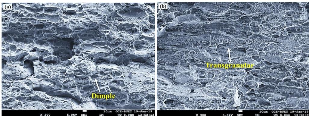
Fig. 6 SEM image of fracture surface along (a) longitudinal-alloy 02, and (b) transverse directions-alloy 02 as-aged at 120°C/24hr
