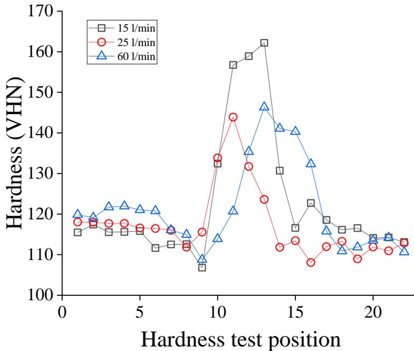
Figure 3. Hardness profile on welded joints
