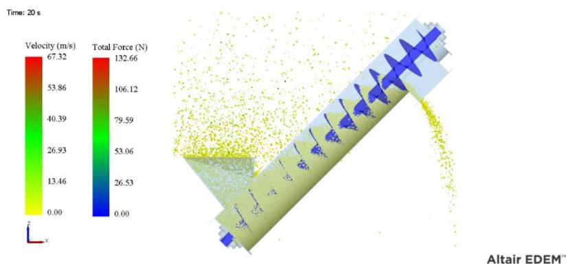
Figure 3. Simulation on 45 Degree modelling with 50 Rpm
