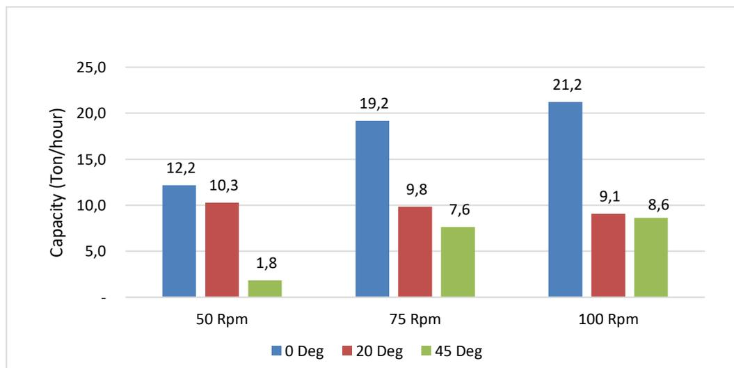
Graph 3. DEM Simulation results for capacity
