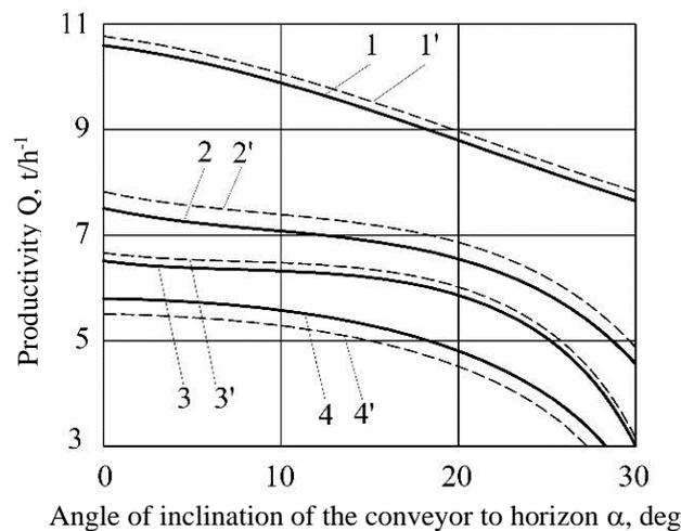
Graph 5. Productivity  $Q$  of the conveyor with a screw working body (solid line) and bladed one (dashed line) at 300 rpm (1 – sand; 2 – peas; 3 – wheat; 4 – corn).
