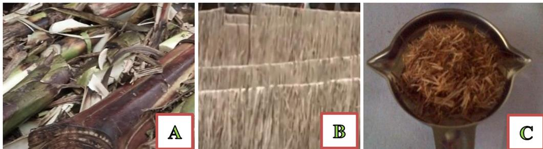
Figure. 1. Banana stem fiber. (a) Banana stem; (b) BSF fiber; (c) NaOH Treatment
