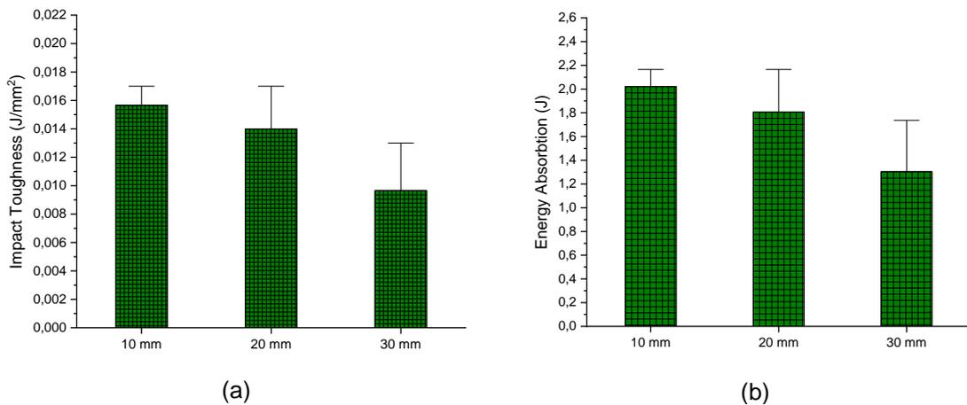
Figure 4. (a) Impact Toughness; (b) Energy Absorption
