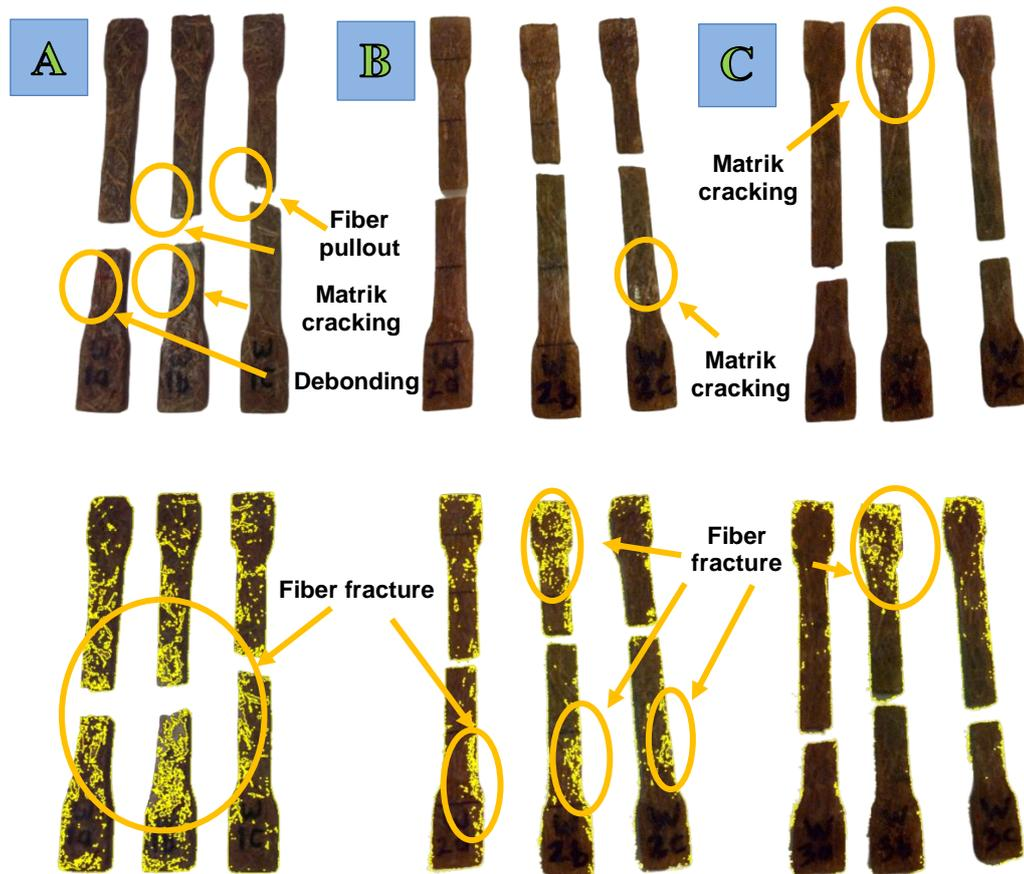
Figure 8. Fracture analysis using imageJ. (a) fiber length 10 mm; (b) fiber length of 20 mm; and (c) fiber length 30 mm
