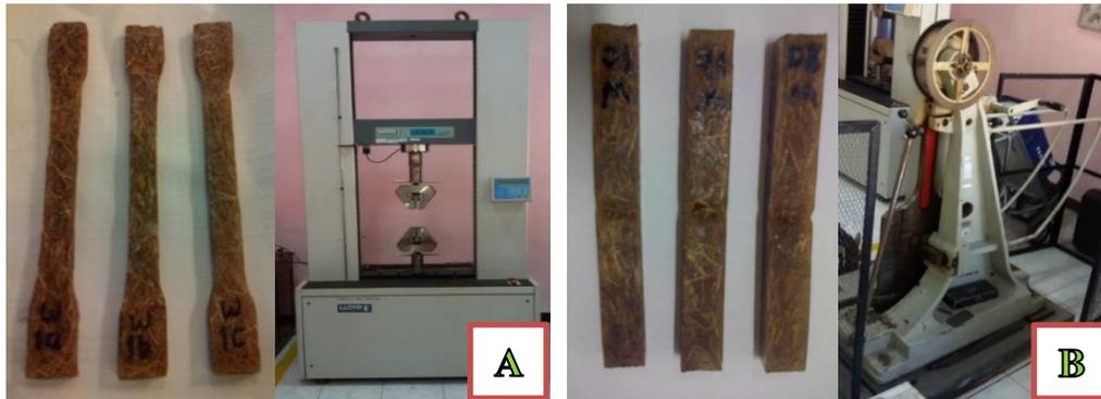
Figure 2. Composite Tests and Specimens (a) Tensile and Flexural (b) Impact Test
