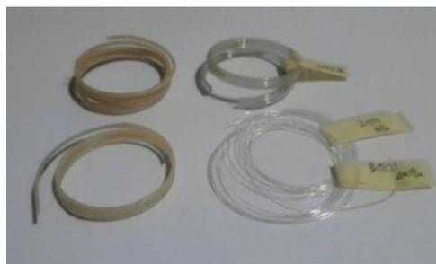
Figure 3.3 Filament produced from the mini extruder
