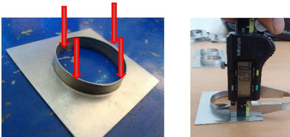
Figure 2.5 Measurement scheme.
