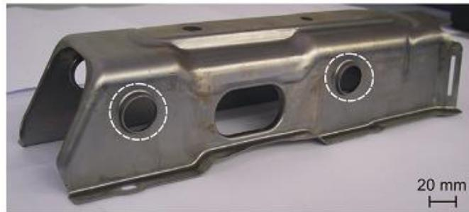
Figure 1.1 hole with outward collar in almost closed surface.
