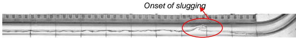
(c) Slug flow pattern for  $J_G=2.47$  m/s and  $J_L=0.020$  m/s
