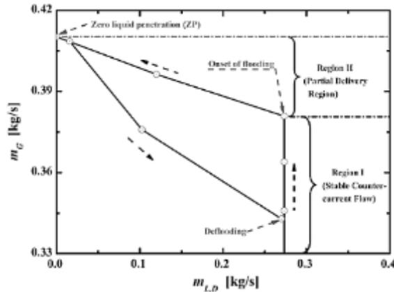
Figure 2.1 Terminology of two phase counter-current flow of gas-liquid (Deendarlianto et.al. [2])
