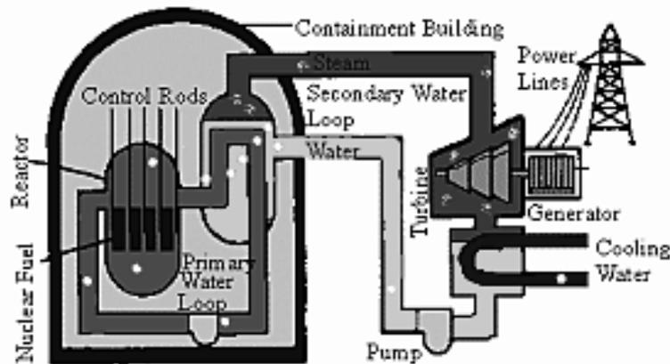
Figure 1.1 Scheme of Pressurized Water Reactor
