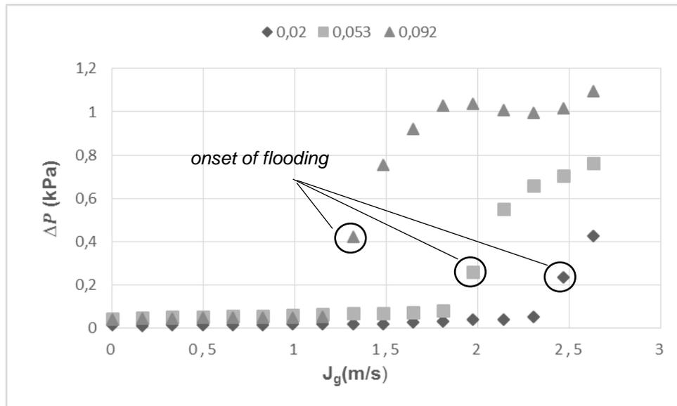
Figure 3.3 Relationship between averages of pressure drop ( $\Delta P$ ) with air superficial velocity ( $J_G$ )
