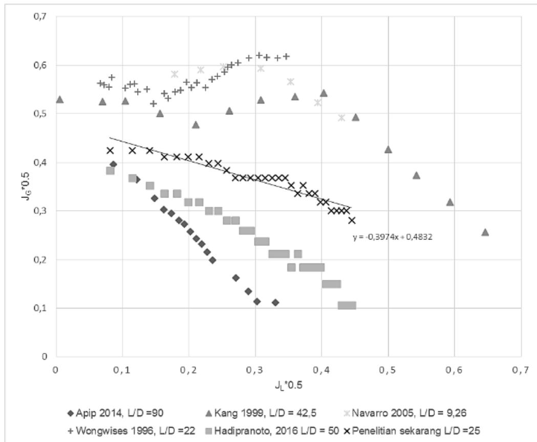
Figure 7 Comparison of onset of flooding curve
