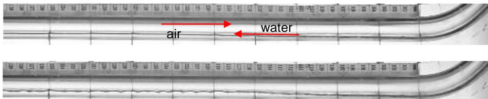
(a) Stratified flow pattern for  $J_G=0$  m/s and  $J_L=0.020$  m/s
