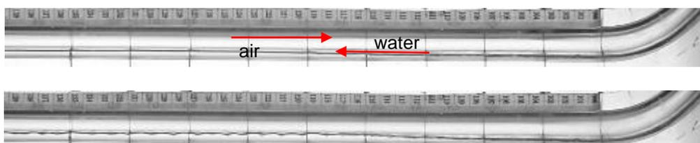
(b) Stratified-wavy flow pattern for  $J_G=1.97$  m/s and  $J_L=0.020$  m/s
