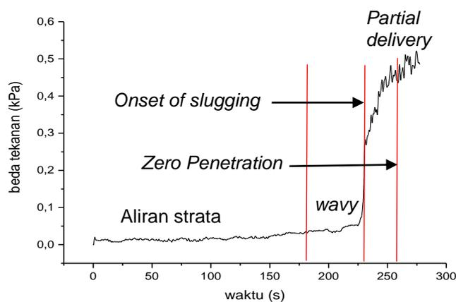
Figure 3.2 Relationship between pressure drop and time for  $J_L=0.02$  m/s
