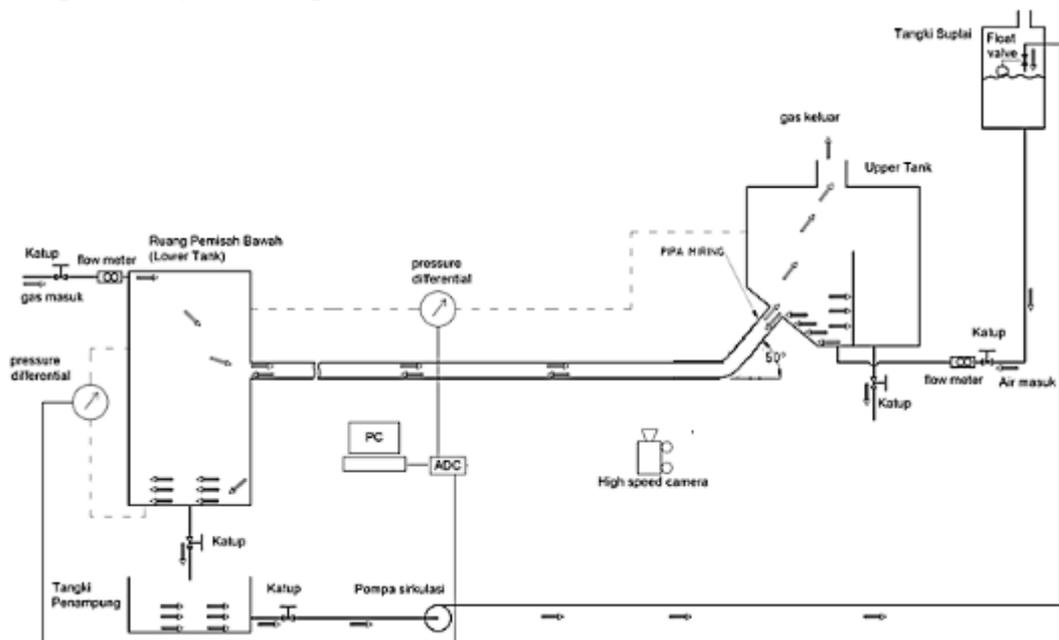
Figure 2.2 Scheme of experimental installation
