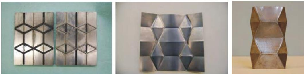
Figure 1.1 Building Origami Crash box with stamping method [9]
