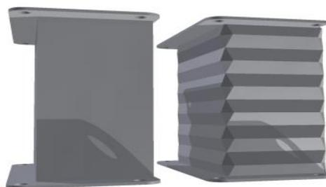
Figure 2.3 Prototype of crash box
