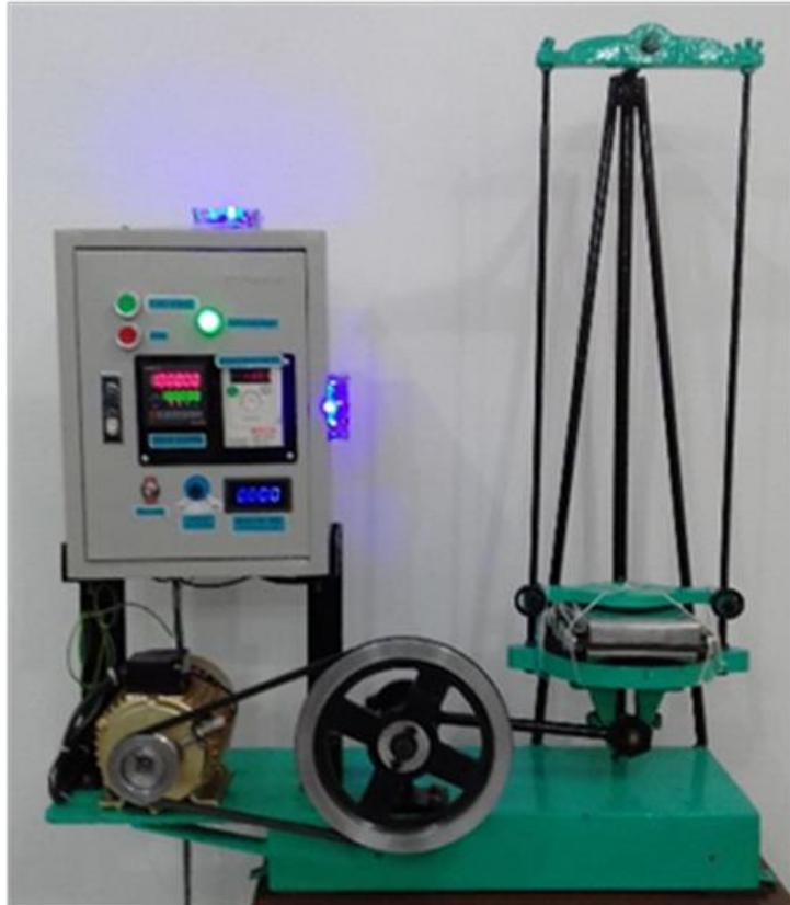
Figure 2.1 Shaker type of HEBM used in this research
