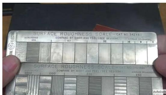
Figure 2.3 Surface Roughness Scale
