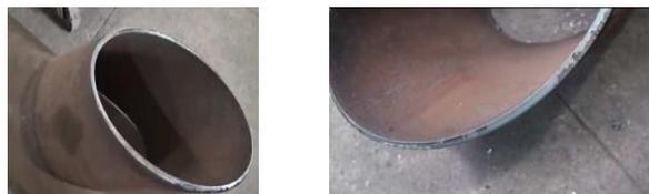
Figure 3.5 Cutting result with 44 mm gap
