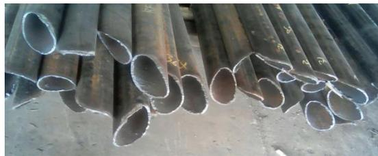
Figure 3.1 Cutting result with 30 mm gap
