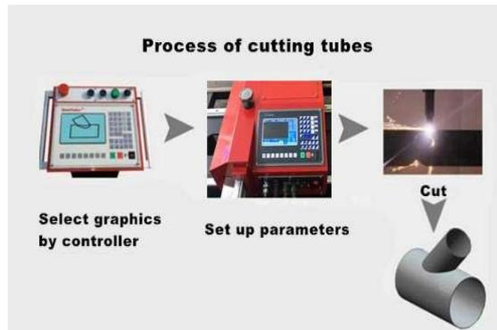
Figure 2.1 Process of cutting pipe
