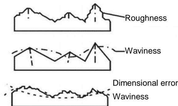
Figure 1.2 Roughness, waviness, and dimensional error of surface
