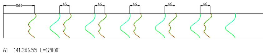
Figure 3.6 Variation gap design of 46 mm
