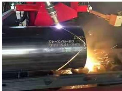
Figure 2.2 CNC pipe cutting process with torch
