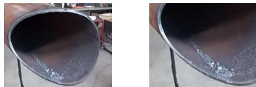
Figure 3.3 Cutting result with 42 mm gap
