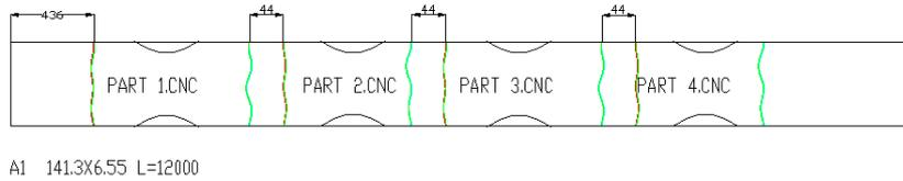
Figure 3.4 Variation gap design of 44 mm
