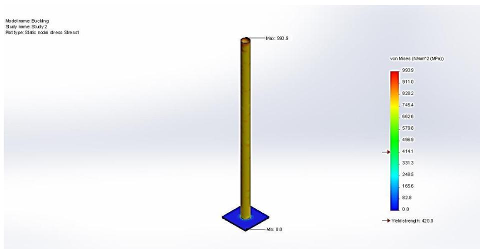
Figure 10. Stress Simulation Result of Construction Steel by Using Solidworks
