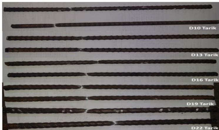
Figure 5. Pull Fin Reinforcement Steel Tensile Test Results
