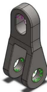
*Figure 7. Swing Hanger Modeling by Using Solidworks*
