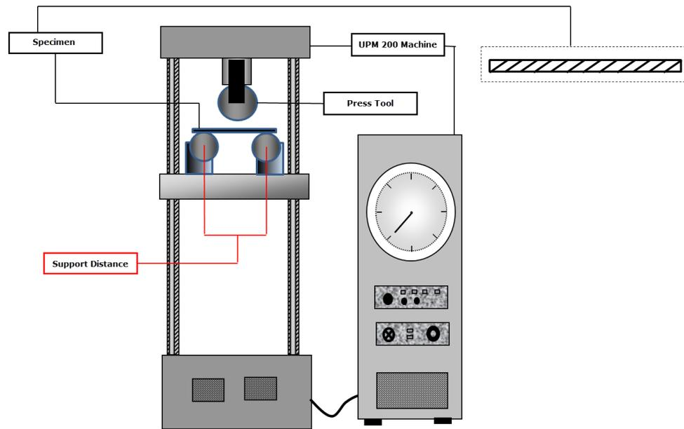
Figure 3. UPM 200 Bending Testing Machine Series
