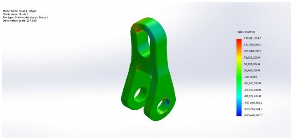
Figure 8. Shear Stress Simulation Result by Using Solidworks
