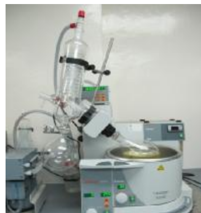
Figure 4. Rotary Evaporator Containing the Extract Solution
