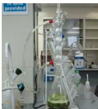
Figure 2. The Design of the Reflux Containing the Gotu Kola Fresh Leaves
