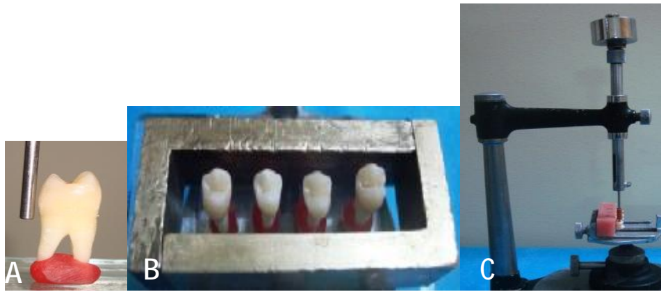
Figure 1: A , Fitting the tooth with a sticky wax and oriented so that the middle third of lingual surface is made parallel to the analyzing rod of surveyor. B , two L-shaped metal plates placed around the teeth. C , load placement over each button.
