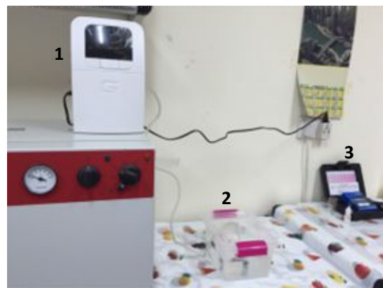
Figure 2: shows the: 1) Ozone Generator 2) plastic container 3) CHE Mets Kit
