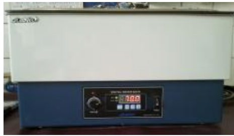
Figure 5: Electronic water bath machine with its control panel.
