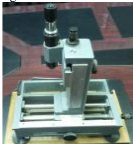
Figure 3: Travelling microscope used to determine dimensional changes.
