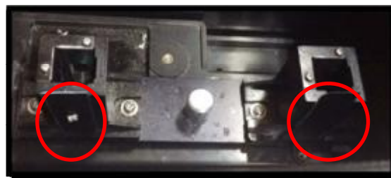
Figure 3: The bracket positioned on the analytical beam holder of the spectrophotometer and the blank on the other analytical beam holder.
