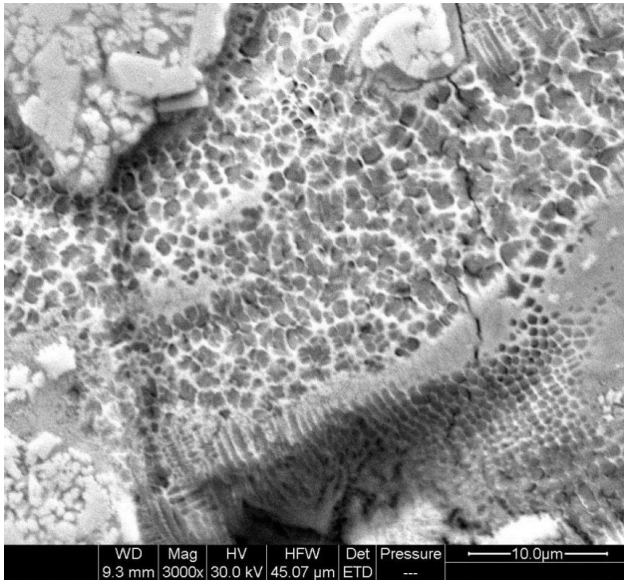
Figure 3. SEM image of laser modified HVOF thermally sprayed Inconel 625 and WC-12Co coatings; laser power 55 W laser scan speed = 1250 mm min -1 nanostructured powder
