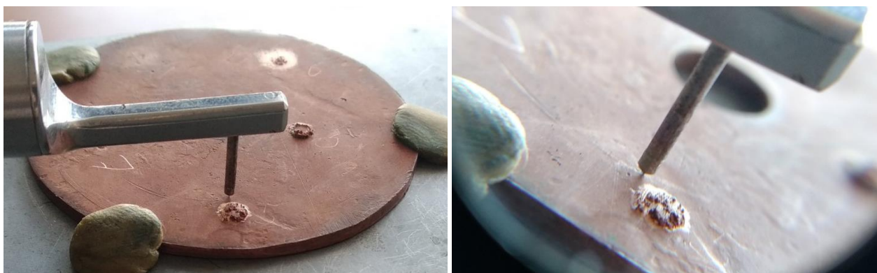
Figure 4. Locally deposited copper on the surface of copper plate during 3D-profilometry
