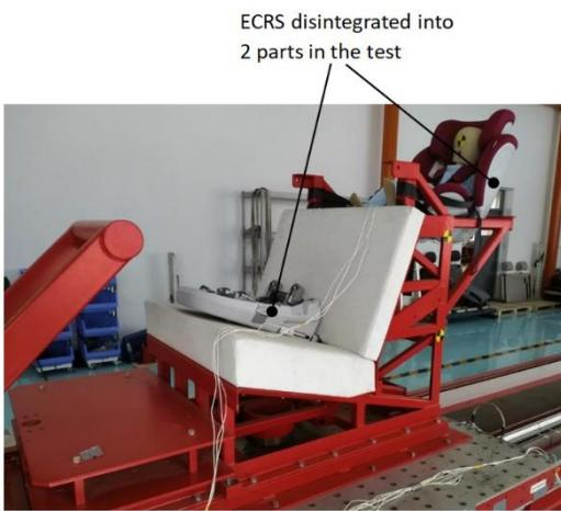
Fig. 11. Damaged ECRS in the fourth test
