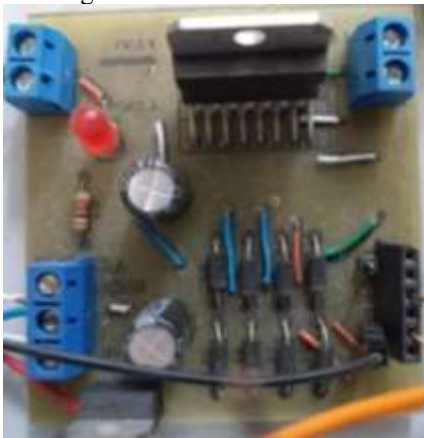
Figure 9. Motor driver (L298N H-bridge).
