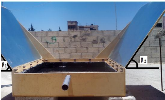
Figure 5. Photographic of Locally Fabricated SSP
