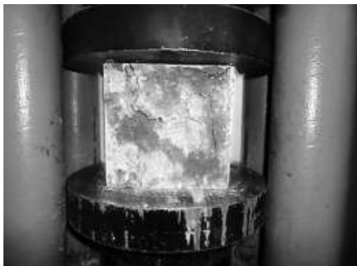
Figure 10 Mode of Failure and Crack Pattern of HSC Specimens with 0.6 Fiber Percentage.
