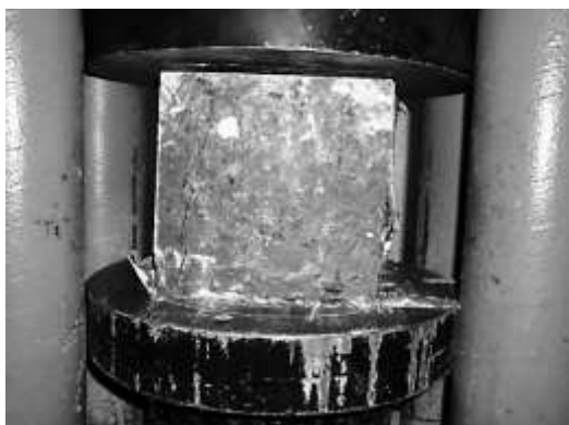
Figure 11 Mode of Failure and Crack Pattern of HSC Specimens with 0.9 Fiber Percentage.
