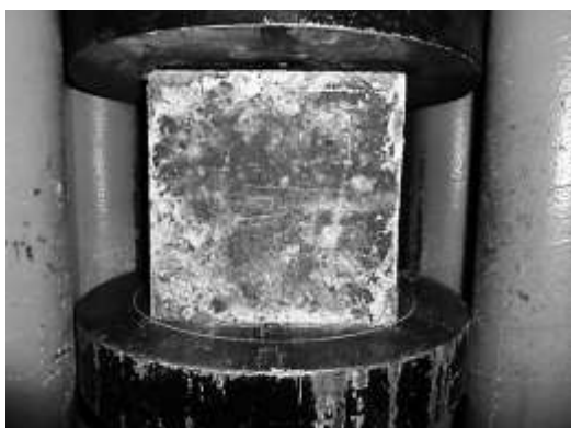
Figure 12 Mode of Failure and Crack Pattern of HSC Specimens with 1.2 Fiber Percentage.
