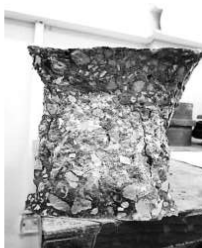
Figure 9 (a) and (b) Mode of Failure and Crack Pattern of HSC Specimens with 0.3 Fiber Percentage.
