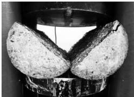
Figure 16 Mode of Failure of Plain HSC Specimens (Without Fiber).
