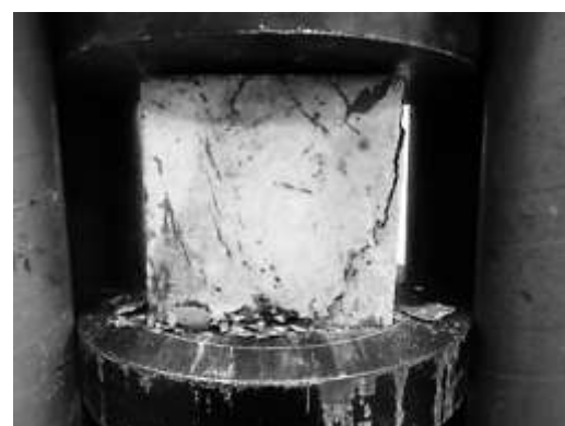
Figure 8 Mode of Failure and Crack Pattern of Plain HSC Specimens (Without Fiber).
