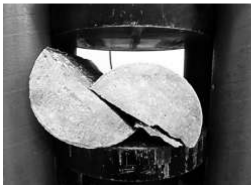
Figure 17 Mode of Failure of HSC Specimens with 0.3 Fiber Percentage
