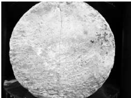
Figure 20 Mode of Failure and Crack Pattern of HSC Specimens with 1.2 Fiber Percentage.
