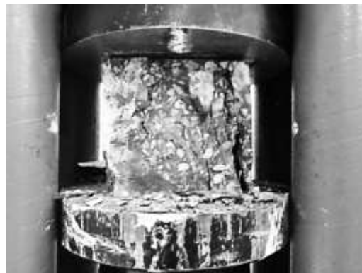
Figure 8 Mode of Failure and Crack Pattern of Plain HSC Specimens (Without Fiber).
