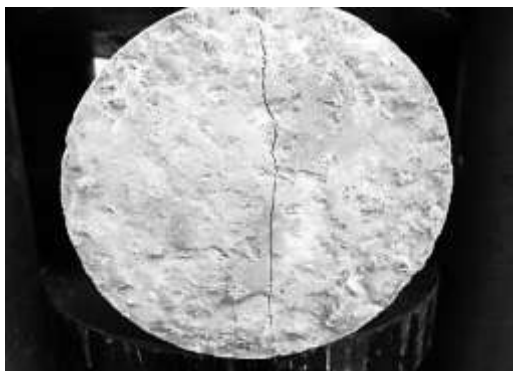
Figure 19 Mode of Failure and Crack Pattern of HSC Specimens with 0.9 Fiber Percentage.
