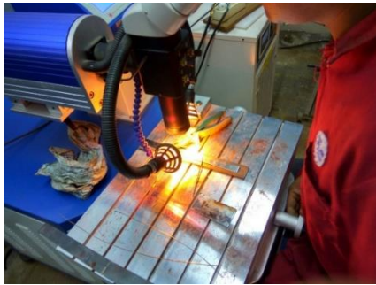
Figure 5. Laser welding process using a laser welding machine
