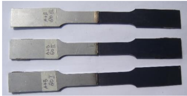
Figure 6. The result of the lasers on dissimilar metal joints
